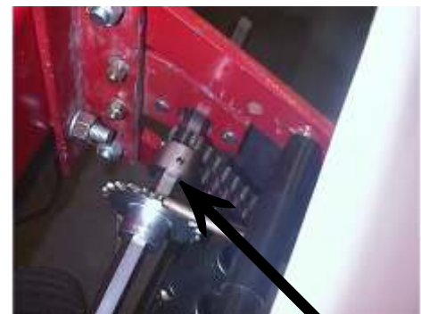
Step 3 Remove sprocket place lock collar ahead of sprocket replace sprocket
