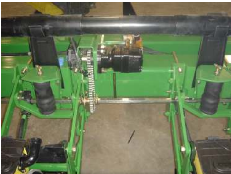
Original position of motor on a Deere planter
