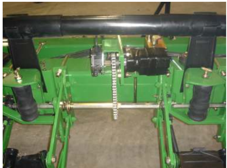
Move the motor to the EXACT center of the section you wish to control
